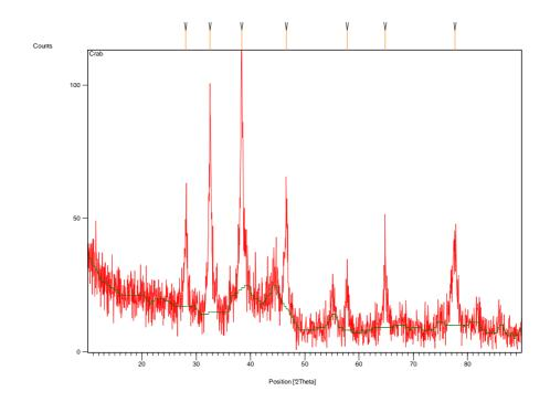
Fig 5. XRD pattern of silver nanoparticles
