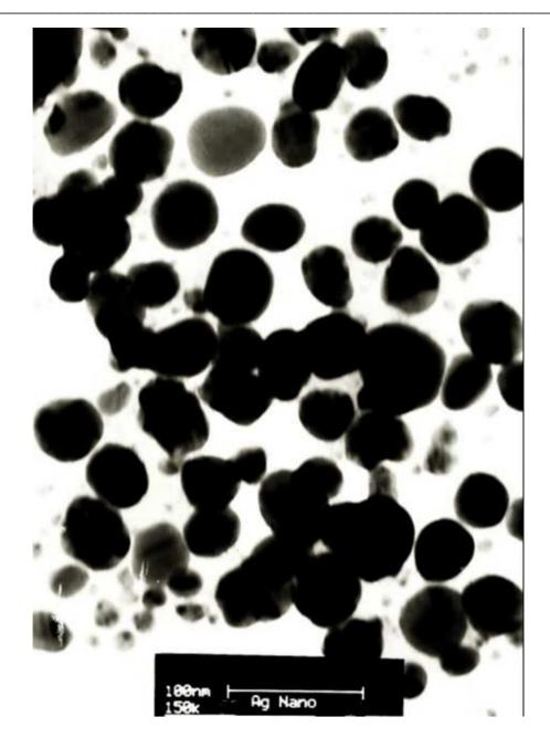
Fig 2. TEM of Silver nanoparticles
